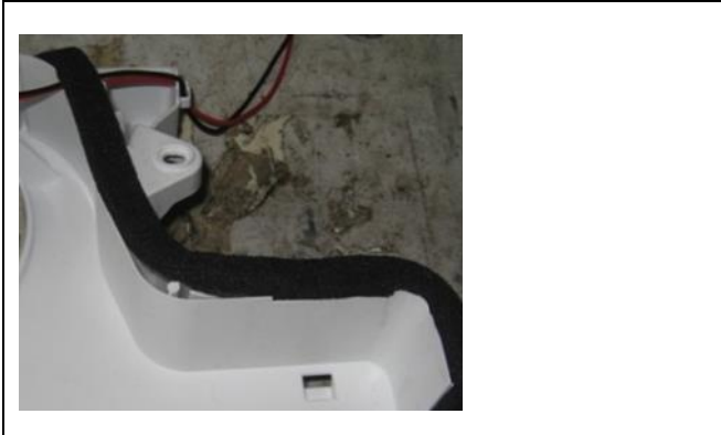
Gasket not aligned with the air channel.
