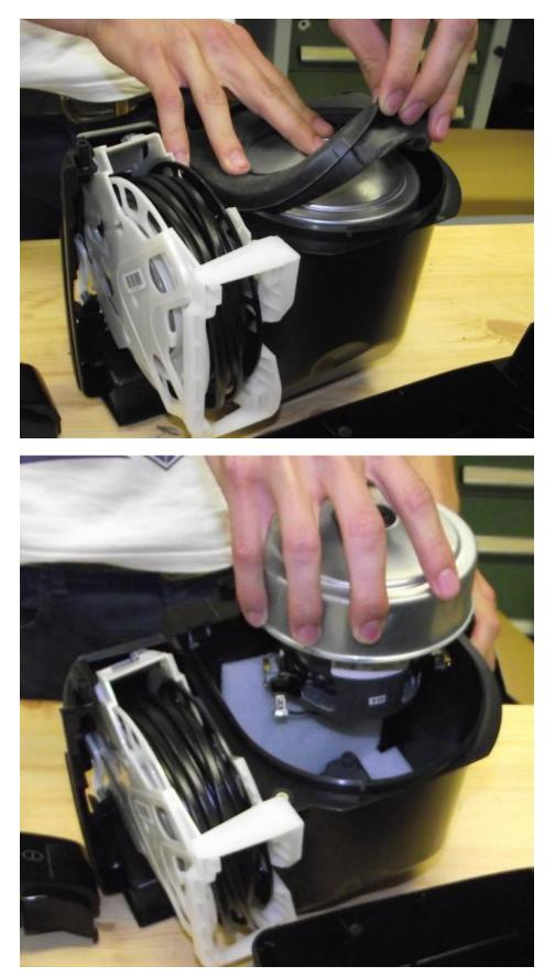
For removing the cord winder the following steps needs to be done:
