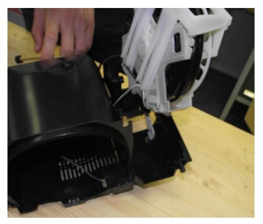
At the end power regulator and PCB are easily removeable.
