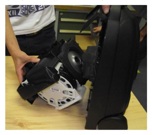
By holding the base carefully pull out the motor housing:
