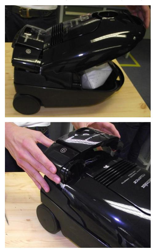
After this move open the dust bag cover to remove the control panel easily.
