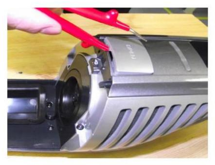
For pulling out the battery holder remove the screws and puff of the plastic:
