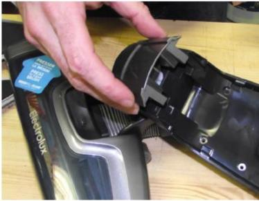
Lift the boss with one hand and release the snappers on both sides to remove it.
