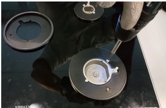
1. Unscrew screws holding old cover to hob
