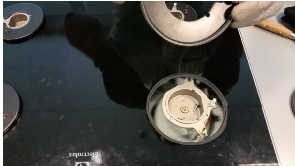
5. Replace the old cover by the new one using gasket according to spare part list for proper type of burner
