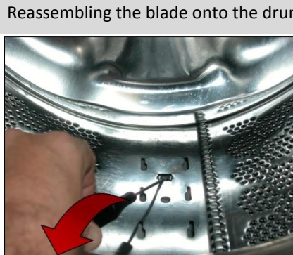
Reassembling the blade onto the drum. Before securing the new blade insert a flat-tip screwdriver beneath the lock tabs and raise them a little.
