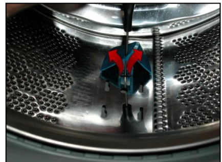
Position the new blade inside the drum guides. Push it towards the back.
