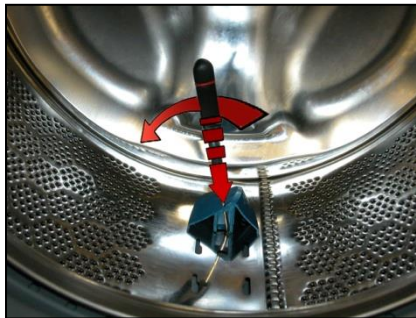
With the screwdriver tilted towards the left push the right-hand tab down.
