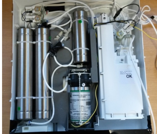
10. Connect the hydraulic fittings to the pump and mount it in its intended position. Route the wires according to the image and connect fastons to the piggy back connectors of the inlet valve.
