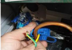
Unplug the connecting wire of the PTC starting relay and of the overload protector
