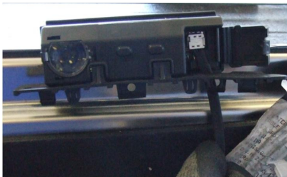
7. Connect the new BOF unit and close the cover.
