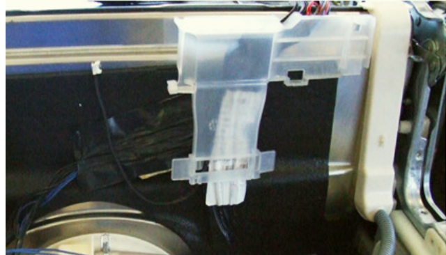
6. Place the BOF harness in right plastic protection. Verify correct positioning of the cable.
