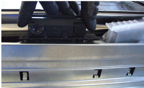
8. Snap in the new BOF in the centre of lower traverse.
