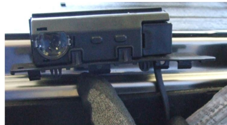
6. Place the BOF harness in right plastic protection. Verify correct positioning of the cable.
