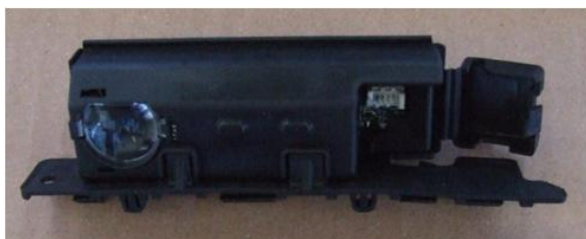
Beam-On-Floor (BOF) display electronics 1119557039
