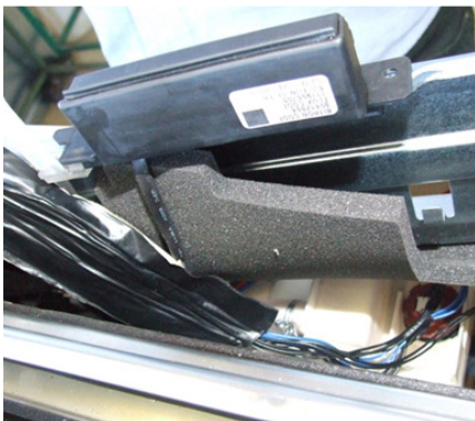
10. Correct positioning of the BOF harness – cable should be placed above the sponge to avoid wear and tear.
