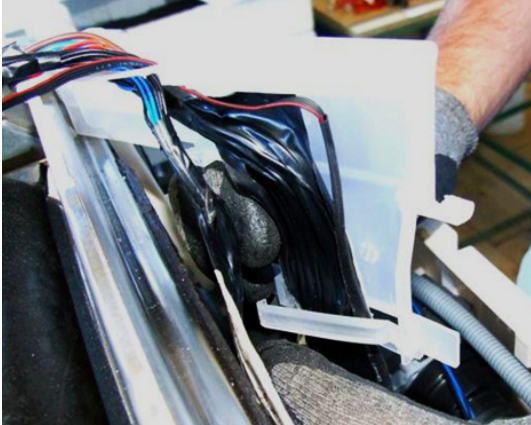
6. Place the BOF harness in right plastic protection. Verify correct positioning of the cable.
