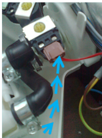
Water drip tray area.
