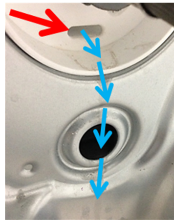
Leakage through back side of appliance.
