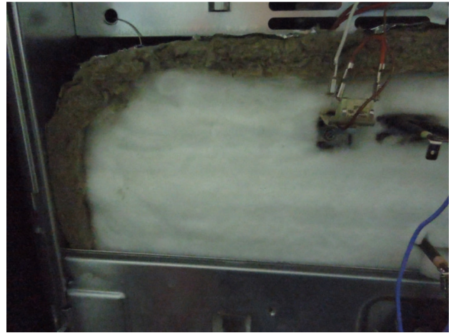
2.5. Correctly laid out insulation
