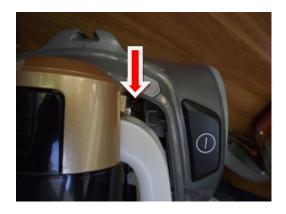
Remove screw and use the screw driver to remove the display support
