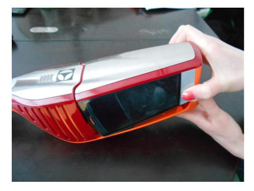
Push the knobs on both sides of the dust compartment and pull it out:
