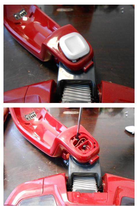
Remove the screws from the back of the base and separate the base part and the top part of the body:
