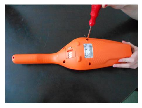
To pull of the pcb remove 2 screws:
