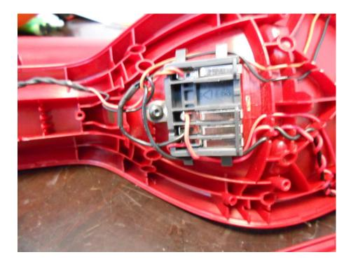
To disconnect the wires push the locking ring and pull of the wires:
