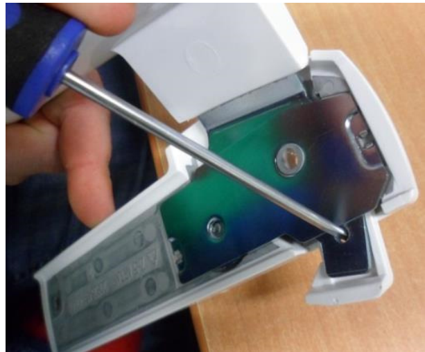
2. Push out the shoe using screwdriver or other pointed hand tool.
