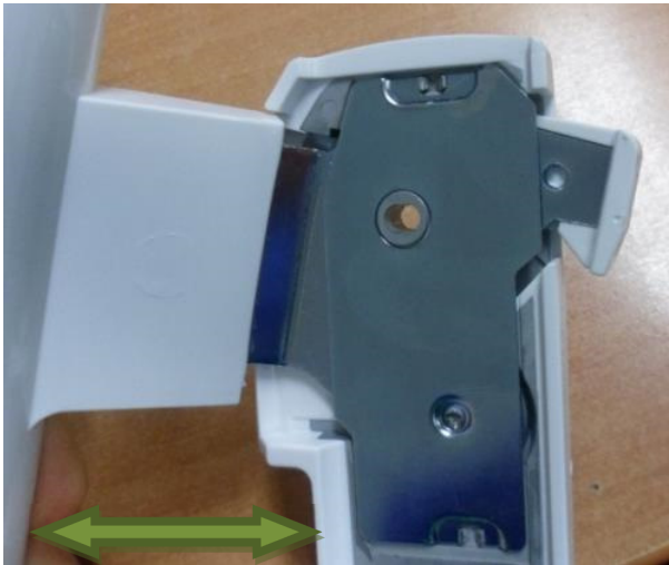
1. Pull the handle and keep in 'open' position during shoe replacing.
