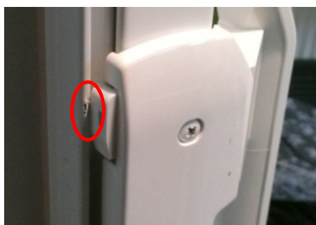
Door gasket damaged by protection shoe.
