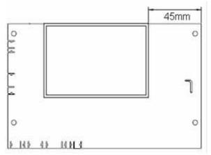
Foil should be placed on the bottom side of the board, 45mm from the edge, as seen on pictures above
