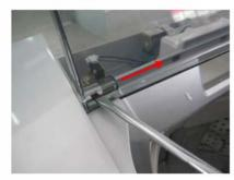
Open the washer lid, move the hinge shaft on the washer lid with slotted screwdriver, then remove the washer lid.
