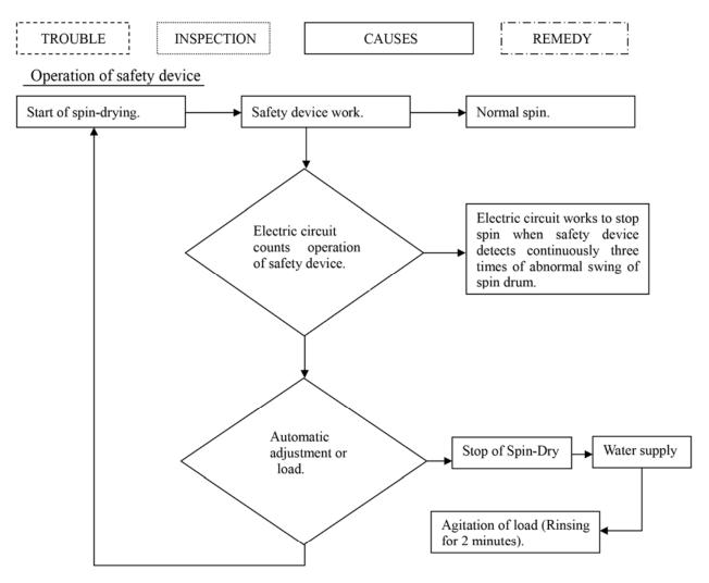
When the safety device works by abnormal swing of spin drum, machine works automatically to stop Spin-Dry cycle and operates water supply valve to pour water into the Wash/Spin Tub and then starts washing cycle for replacing washing clothes evenly.
