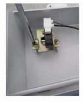
Use cross-style screwdriver to demount the two screws fixed on the safety device switch, pull out the jack, draw the safety device switch out from the slot.
