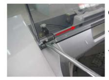
Open the washer lid, move the hinge shaft on the washer lid with slotted screwdriver, then remove the washer lid.
