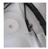
Use cross-style screwdriver to demount the special screw fixed on the reed switch, pull out the jack, then the reed switch can be removed.
