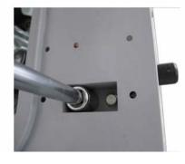
Use the sleeve spanner to demount the two screw assembly under the leg, pull out the pump wire assembly, then the pump can be removed.
