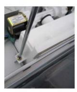
First draw out the detergent tray, then use cross-style screwdriver to demount the two screws fixed on the pour inlet assembly, pull out the jack, draw the pour inlet assembly from the step surface.
