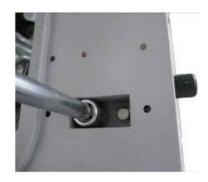
Use the sleeve spanner to demount the two screw assembly under the leg, pull out the pump wire assembly, then the pump can be removed.
