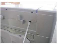
First use cross-style screwdriver to demount the two screws fixed on the back plate.
