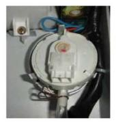
Warp the fastener on the top plate, pull out the jack and air trip hose, then draw the water level sensor out from the top plate.
