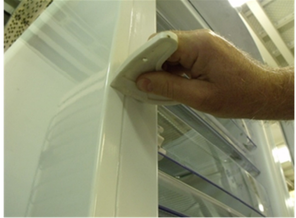
4. Push the silicone into the gaps using plastic tool.
