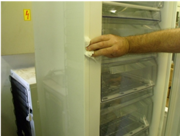
1. Clean up all surfaces around inner liner and housing interlink.
