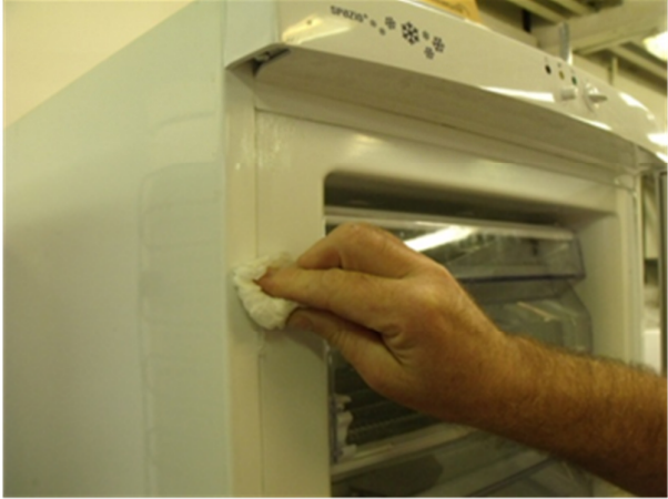
3. Remove excess of silicone using wet paper towel or textile.
