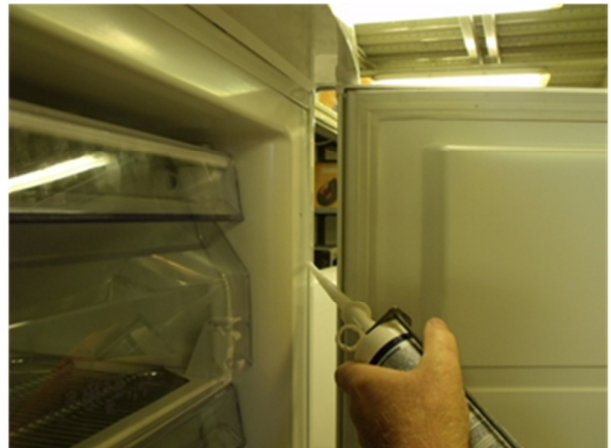
2. Fill up the gap around inner liner with silicone.
