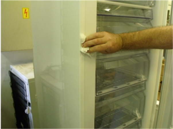
5. Clear remaining silicone from flat surfaces using dry paper towel or textile.
