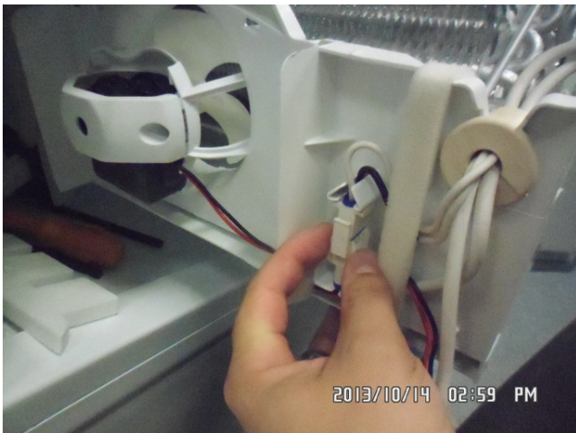
14. Unplug connectors as shown on pictures above. IMPORTANT: Connect brown+blue wires from thermal cut-out to white+black wires from defrost heater.
