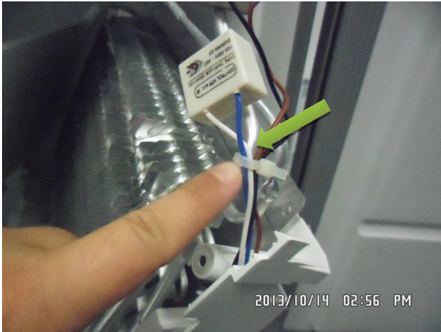
13. Cut off cable clamps. IMPORTANT: Be careful not to damage wires.
