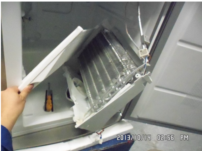
11. Remove EPS insulation.
