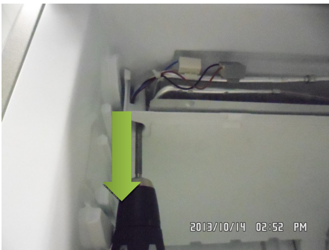
5. Remove evaporator battery fixing screws.
