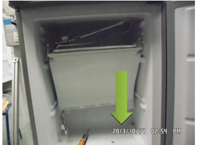
8. Bend the back side of evaporator battery down.
