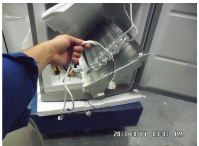
16. Remove faulty thermal cut-out.
