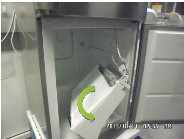
9. Turn the left side of evaporator battery to front and right side.
