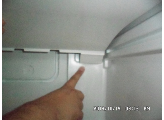
28. Insert the drain outlet into drainage hole.
