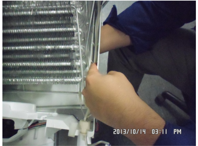
22. Insert cables into cable channel.
