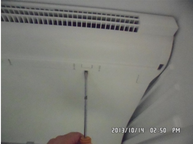
31. Assemble evaporator grid onto module.
