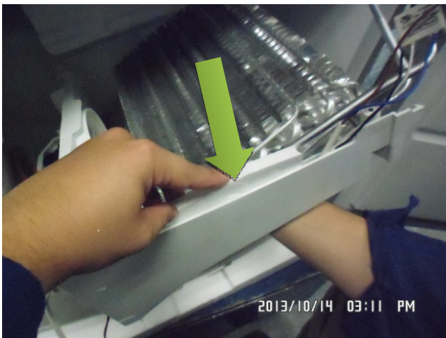
23. Put back side EPS insulation.
