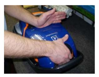
Display cover is easily removable with the help of a thin tool:
