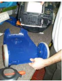
For handle removing take out the screws and with the help of a nozzle disjoin the parts (both sides):
