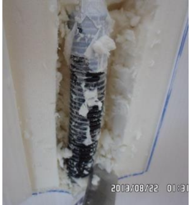
4. Remove foam from around the drain hose. Note: Be careful not to damage inner liner.
