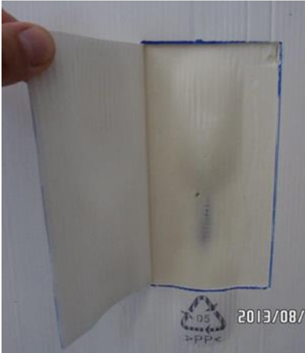
3. Cut corrugated material following markings and bend out to the uncut side.
