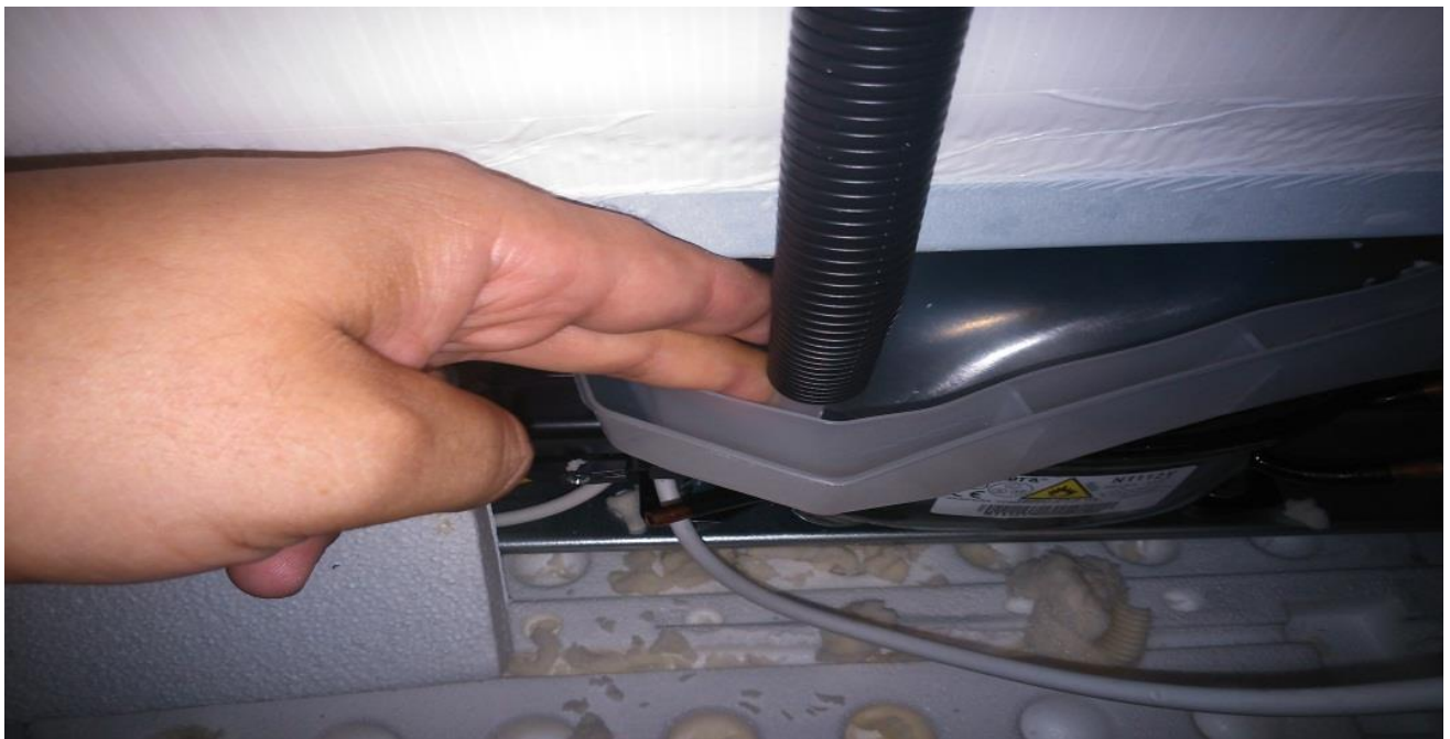
13. Cut hose to required length and insert the end into evaporation tray. Note: Make sure it stays in tray and tray is secured on the compressor.
