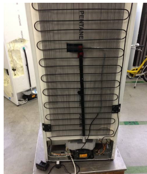
10. After positioning the heating element, remove the metal sheet and fix the cable to the corrugated material with adhesive tape
