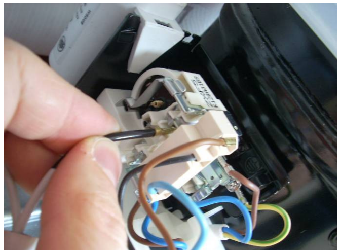
3. Remove the fastening screws from the fastons on the blue and brown wires
