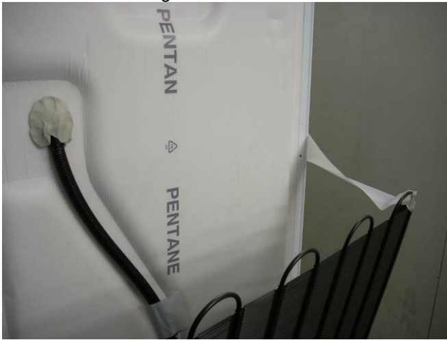
1. Unplug the appliance. Remove the condenser screws and secure it to the cabinet using adhesive tape.
