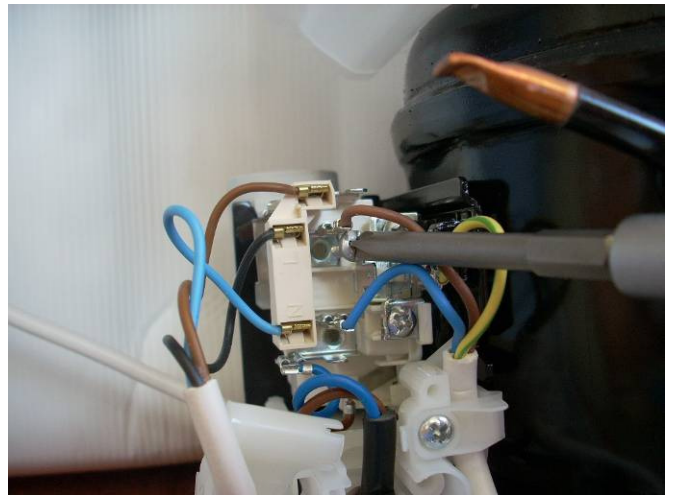
3. Remove the fastening screws from the fastons on the blue and brown wires
