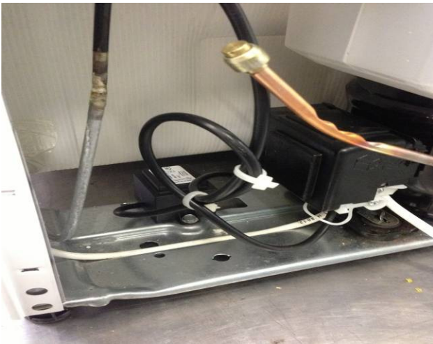
10. Secure the transformer cable with clamps
