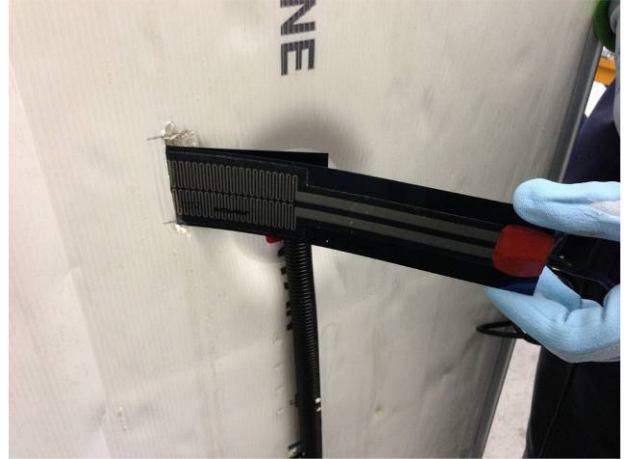
8. Slide the metal sheet with heating element above the other one
