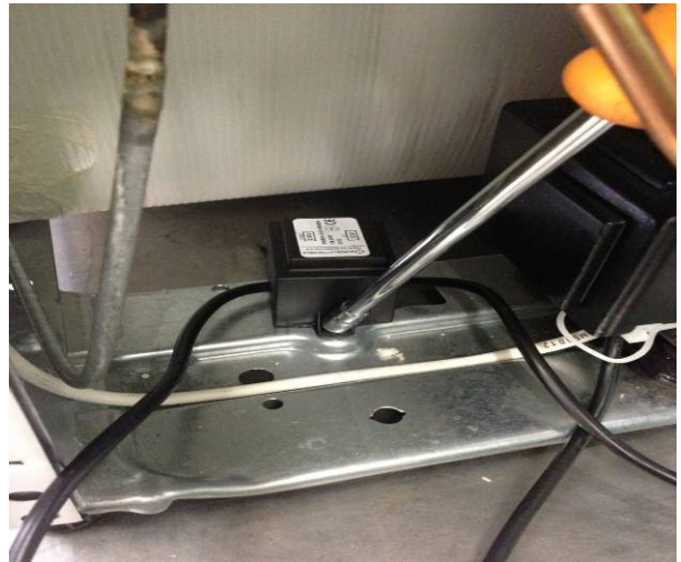
9. Fix the transformer on metal cross bar
