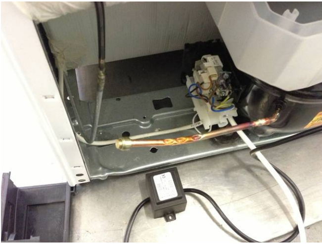
1. Remove the terminal board cover
