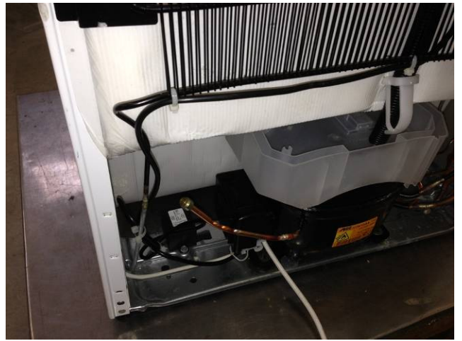
9. Fix the transformer on metal cross bar
