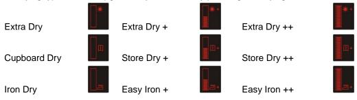
The symbols and the bar graph are only shown in programmes where adjustments are possible. If the drying button is pressed in programmes which do not include this function, the display will show Err.
