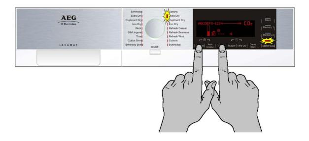
To change the conductivity value according to the table, press the Start/Pause button.
