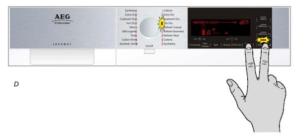
The Demo mode remains enabled even after the tumble dryer has been turned off at the ON/OFF button. When the ON/OFF button is pressed to restart the appliance, the display will show DEM for a few seconds, to facilitate the use of the Demo function in a showroom.
