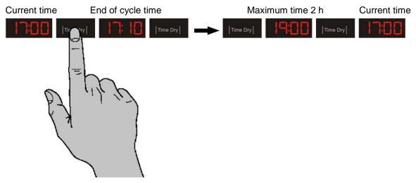
If you reach the maximum time, the line of text will display the message MAXIMUM TIME REACHED and the next step resets the timer to 0 (zero).
