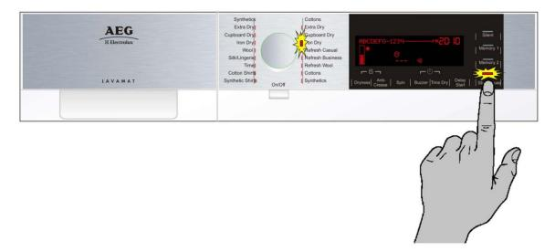
When a programme is selected and the appliance door is closed, simply press the START/PAUSE button to start the cycle.
