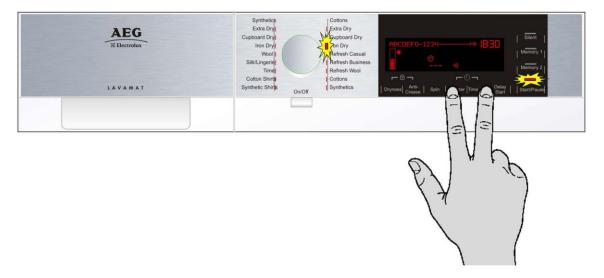
Press the keys **Buzzer and timed drying** simultaneously, the line of text will display the message TIME OF DAY and the hour set will be shown on the right hand digit.
