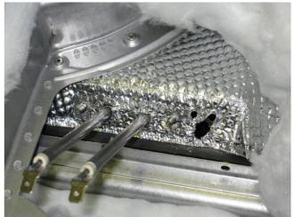
Fix the PT500 sensor on the new **U-flange** (A) and place the new flat plate (B) over the heater connections on the cavity.
