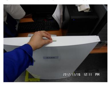
3. Drill the end cap in 30 mm deeply with  $\emptyset 6$  mm spiral drill
