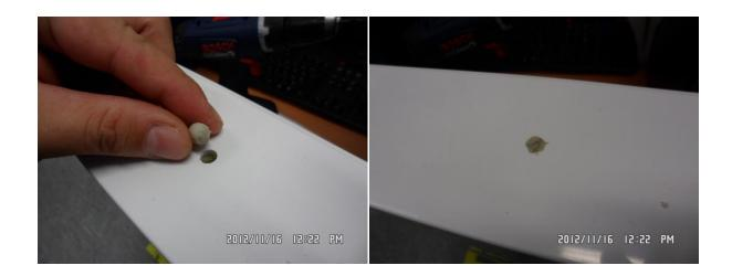
5. Take the magnet into the drilled hole and push until is aligned with the door end cap
