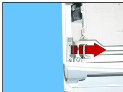
Remove the control panel and position it as shown in the figure, making sure you introduce a protection to prevent scratching it.
