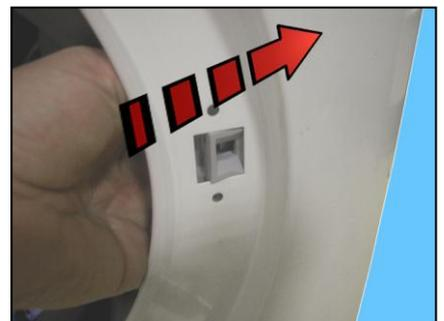
Pull out the wiring protection from the door safety interlock.
