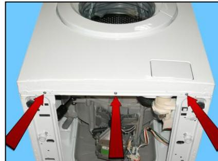
Remove the four screws which secure the front panel to the sides.
