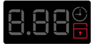
↩ - **Wrong choice of option**, is displayed by Err, when a function not compatible with the chosen programme is selected. The wrong selection is also indicated by an acoustic alarm (if turned on).
