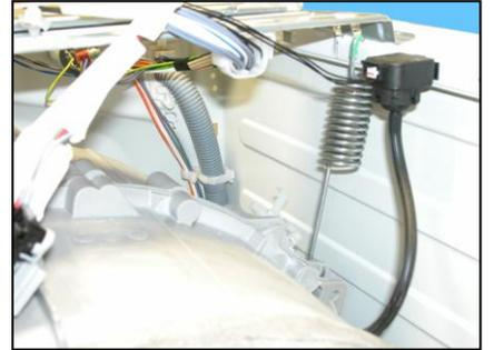
When reattaching the springs (after repair work which required their removal), make sure that the bushings shown in the figure are featured on both ends (the colour of the bushings in the photos below may vary).
