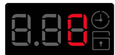
↩ - **Delayed start**, selected via the relevant button. After the START/PAUSE button is pressed, the countdown starts and the delay time decreases hour by hour. In the last two hours it decreases by 30 min. at a time and in the last hour, one minute at a time.
