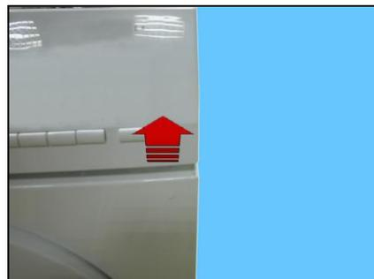
Release the anchor tab which secures the detergent dispenser to the crosspiece.
