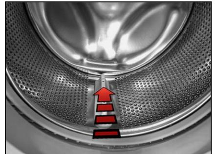
Insert the screwdriver (in the central slot of the left-hand row) at a right angle to the blade, so as to position it at the centre of the two drum tabs.
