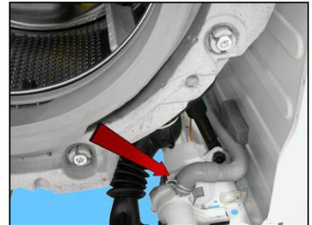
When re-assembling, arrange the pipe in contact with the foam and insert it into the clamps placed there to hold it.
