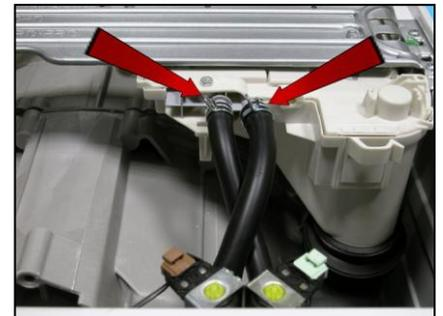
Unfasten the screw in the clamp that fixes the detergent loading pipe to the tray, and remove it from its housing.
