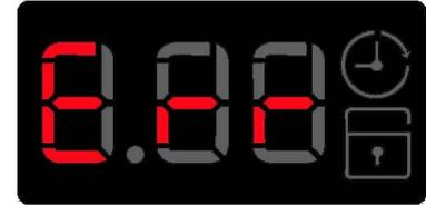
↩ - **An alarm code**, indicates an error in the appliance operation; simultaneously to the displaying of the code on the display, the yellow LED button (above the START/PAUSE button) flashes.
