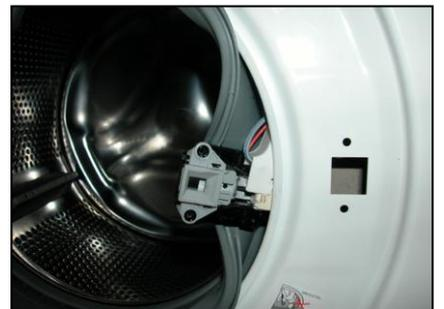
To reassemble the door safety interlock, repeat the same tasks in reverse order.
