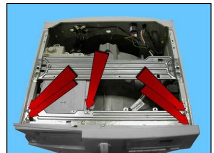
Cut the clamp, unhook the cable from the hook indicated by the arrows.
