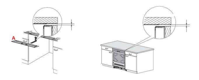
To protect the kitchen worktop, in alternative to the metal steam protection, an "Adhesive Plastic foil" is available. It avoids any kind of disturb signal of the Electronic
