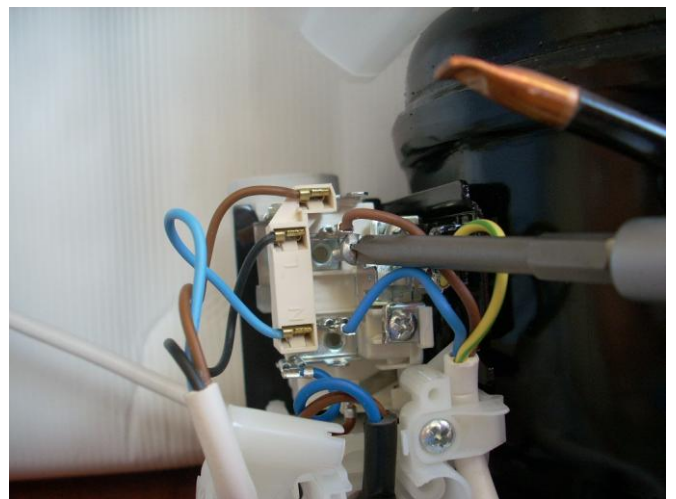
c) Remove the fastening screws from the fastons on the blue and brown wires.
