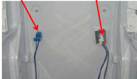
Defrost heater +temp. fuse housing
