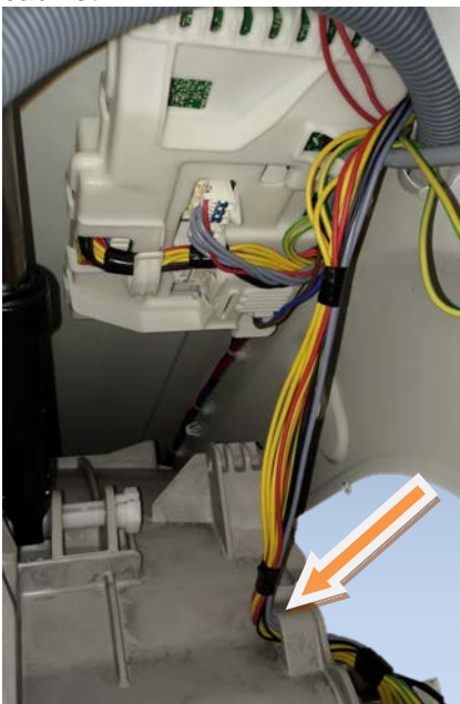
Remove the bundled cables from the hooks that hold them close to the washing group
