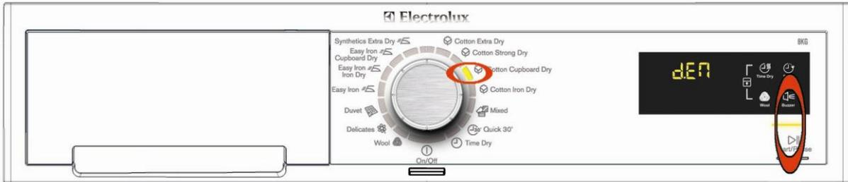
The Demo mode remains enabled even after the tumble dryer has been turned off at the ON/OFF button. When the ON/OFF button is pressed to restart the appliance, the display will show DEM for a few seconds, to facilitate the use of the Demo function in a showroom.
