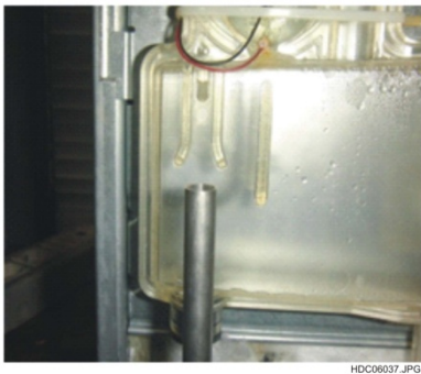
Fig. 12 : Overfilling pipe snap assembly.
