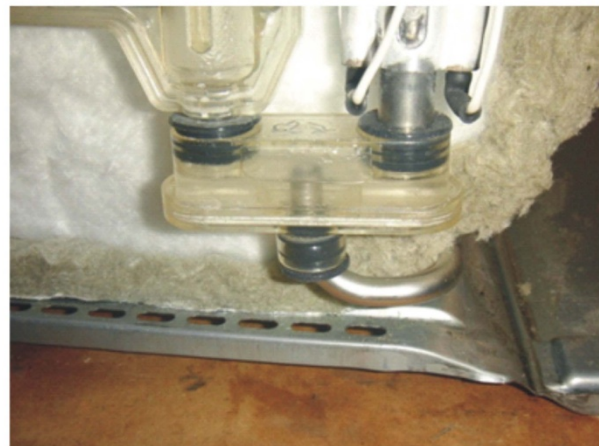
Fig. 18 : Outlet filter detail
