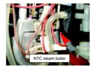
Check both NTC sensor connections on the board for loose connections, check the ohm resistance: if 0 (short circuit) of infinite replace it.
