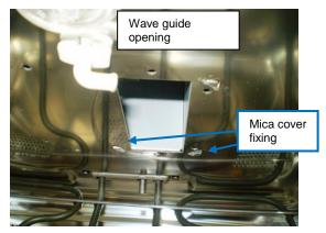
2. Place the new mica cover 50293747007 in the two rear fixing points
