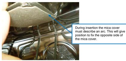
4. Place the mica cover in the front fixing points and perform a visual inspection to verify if the 4 corners are well blocked. Hold the grill heater element in his support.
