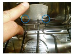
3. Press the mica cover against the fixing point and at same time force the mica cover to obtain an arc in the middle point.
