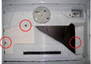
2. Disconnect to evaporator connector. (blue connector)Remove the evaporator by pulling forward in a horizantal direction.Do not push it up or down. You may broke the fixing plastics.
