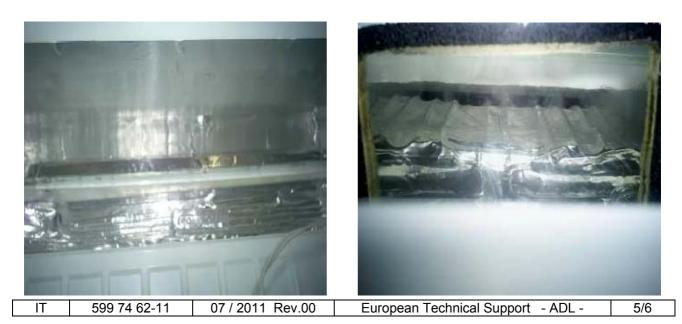
9. Place the finevap to the its place and connect the evaporator connector.
