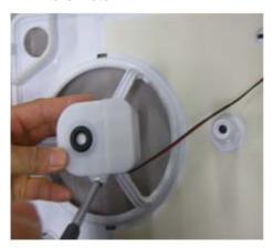
8. Assembly the clamp to the new fan
