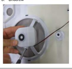
4. Remove the fixture motor
