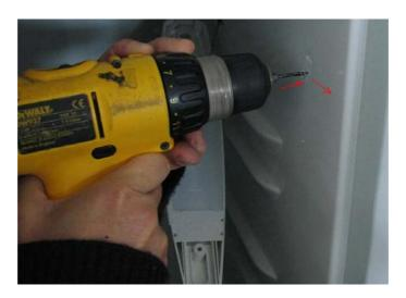
5. Fit into the hole the end of a simple tool (d max. =2.5mm)
