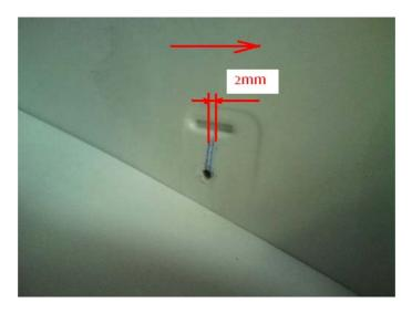
4. With a hand driller (D=3mm) carefully enlarge the hole in the inner liner
