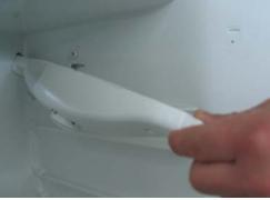
3. Put a mark to the inner liner where to move the light switch (2 mm forward from the original hole position)
