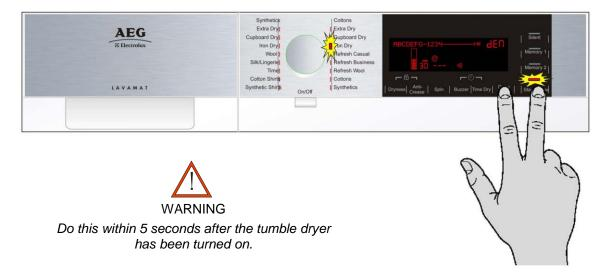
The Demo mode remains enabled even after the tumble dryer has been turned off at the On/Off button. When the On/Off button is pressed to restart the appliance, the display will show DEM for a few seconds, to facilitate the use of the Demo function in a showroom.
