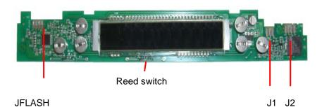
J1: Connection to PB (3wires; only +12V)
