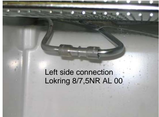
17, Make the Lokring connections in proper way
