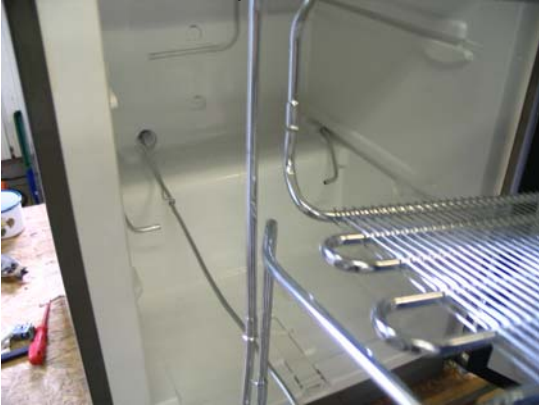
14, Cut the end of evap. tube to Ø8 mm
