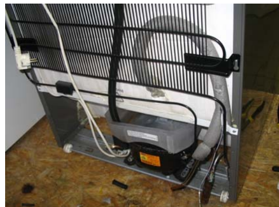
21, Make up the cooling circuit, do the leakage test, evacuate and fill it according the relevant service manuals.
