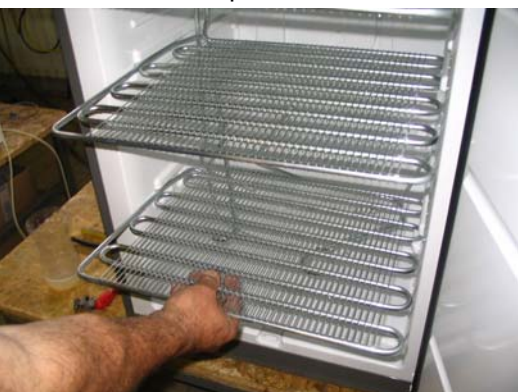
10, Pull out the evaporator from the cabinet
