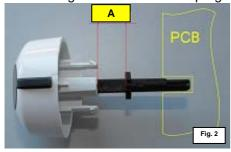
The problem is caused by the excessive distance (A fig 2) between the knob and the retainer ring of the selector pin.
