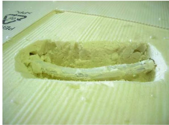
5, Re-insulate the suction tube. Use Armaflex tube (see at the picture) or PUR foam.
