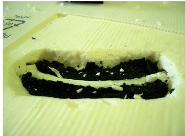
6, Bend back the cartonplast cover and put adhesive foil at the edges. AL adhesive tape is recommended! (at the picture used white plastic tape, this case takes min. 3-4 extra layer).
