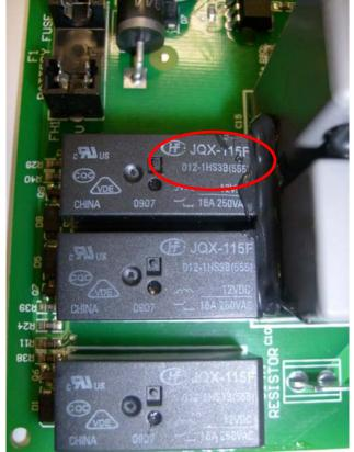
The lettering on the relay "JQX-115F-012-1HS3**B**" shows the wrong relay.
