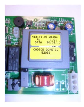
"DATA 20/02/10" is the production date. Electronics produced between 09/12/09 and 20/02/10 could be involved.
