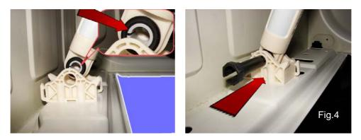
If difficulty is encountered when inserting the pin (fig. 4), apply a small quantity of grease (Cod. 5026 24 16-00/6)
