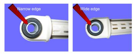
When inserting the damper into its seat (in the lower section of the cabinet or the tub), ensure that the ferrule is correctly positioned. The pin should be inserted from the side on which the lip of the ferrule is wider. The ferrule is available as a spare part (part no. 344 91 25-30/59.
