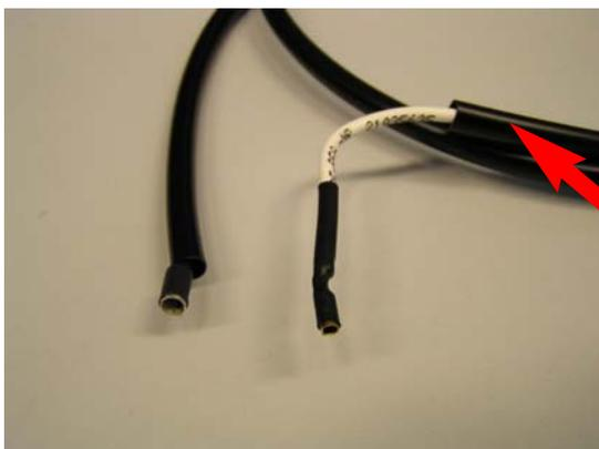
**Insulating tubing for ignition cable 293 5712-01/4**
