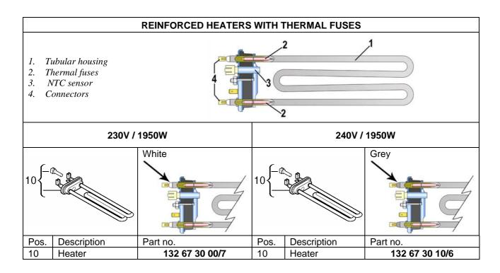
To identify the heater, check the part no. printed on the flange indicated by the arrow (see figure).
