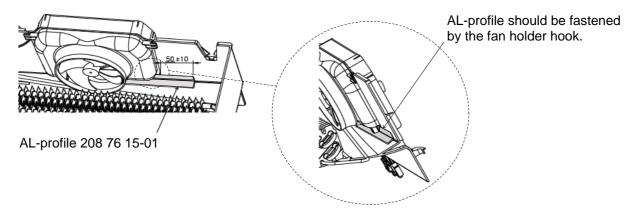
Visualization board according to the spare parts list and the AL-profile 208 76 15-01 can be ordered from Distriparts.
