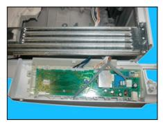
b. Remove the screws and release the hooks which secure the board casing to the control panel.
