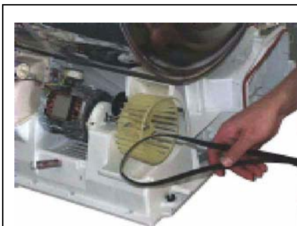
Insert the belt under the fan
