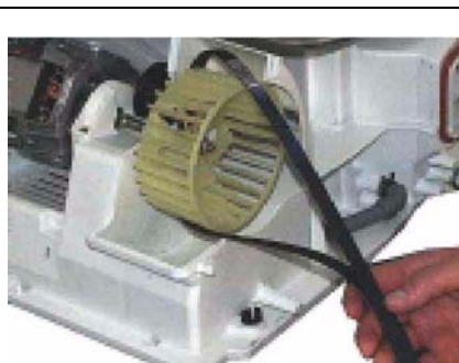
Position the belt on the transmission shaft
